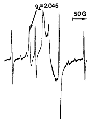
Figure 5. EPR spectrum of used, active MgO(B). The analysis was obtained with the MgO under vacuum at 77 K.
